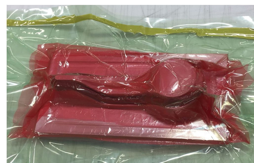
Figure 5. Rail conformed to rail mold shelf inside vacuum bag. Rails were cured in either an oven or autoclave.
